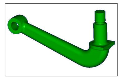
Re-designed arm. Note also the increased corner radius where the shaft meets the flange.
